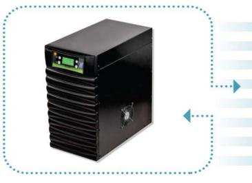
TPS 7.5 KVA/120V Model I/P Range (Normal Mode) 100V-285V+10V I/P Range (UPS Mode) 180V-265V+5V O/P Voltage Battery Mode 220V+10V O/P Frequency Battery Mode 50Hz+0.5Hz O/P Waveform Battery Mode Sine Wave Low Battery Alarm 108V+0.2V Low Battery Shutdown 105V + 0.2V Running Load 48A+2A Overload 50A+2A DC Voltage 120V **Charging Current** 15A+1A Charging Cut off 145V/140V+0.2V No Load Current <2.5A Efficiency >85% Battery Recommended 135AH-300AH
